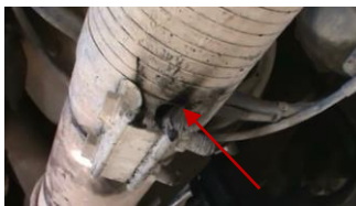
Soot indicating exhaust leak under cab
