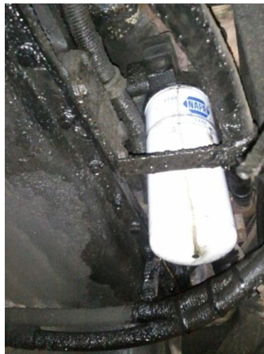
Significant engine oil leak
