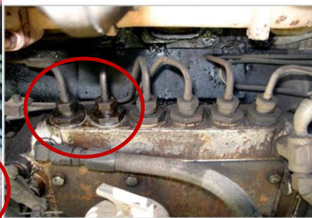
Fuel Leak at Engine
