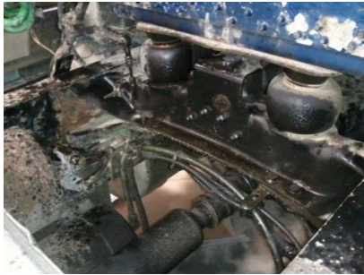
Significant transmission leak
